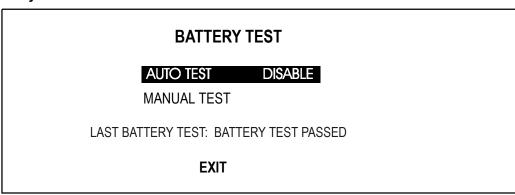
The auto battery self test can be enabled / disabled from the Battery Test Screen. It is performed unattended by programming Time, Date, Test Cycle and Test Duration in Battery Self Test Screen. Selecting MANUAL TEST from the Battery Test screen will perform an Operator-initiated test.
